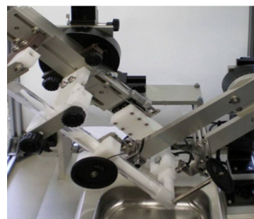
Fig. 3. Micro-feeding of nano particles based on a novel vibration shear flow method.
