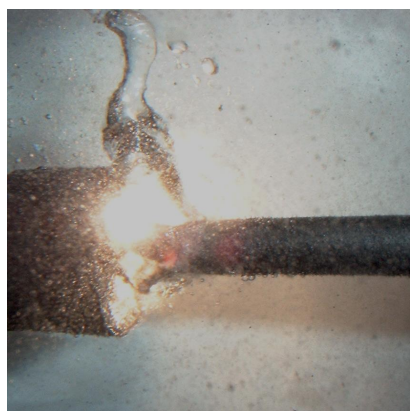
Fig. 2. Photograph of arc plasma in water. This reaction system can enable ones to obtain nanocarbons such as carbon nanotubes, nanohorns, etc.
